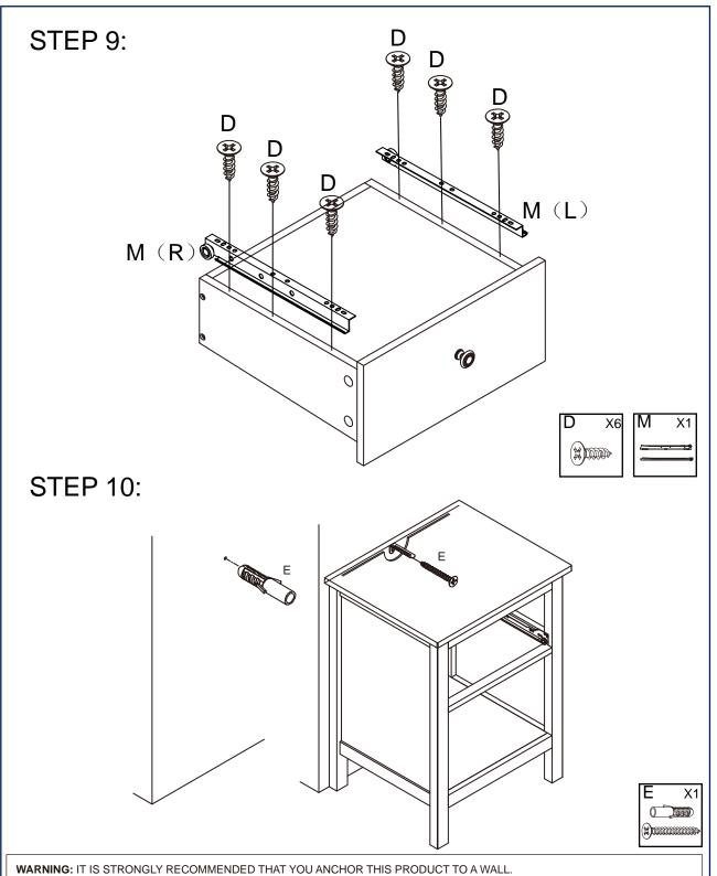
YOUNG CHILDREN MAY BE INJURED OR KILLED BY TIPPING FURNITURE OVER. ALWAYS USE AN ANTI TOPPLE RESTRAINT. This hardware, when properly installed, could provide protection against the unexpected tipping of furniture due to improper use. Please ensure the anti-tipping hardware provided is suitable for your wall or else it might damage your wall during installation. Please refer to page 6 for guidance on suitable wall fixings.
